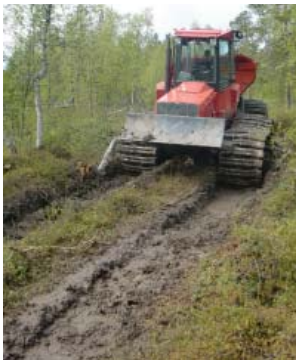
Figure 14, 15,16 Deep ruts from heavy vehicles can be avoided by placing logs in the track.
