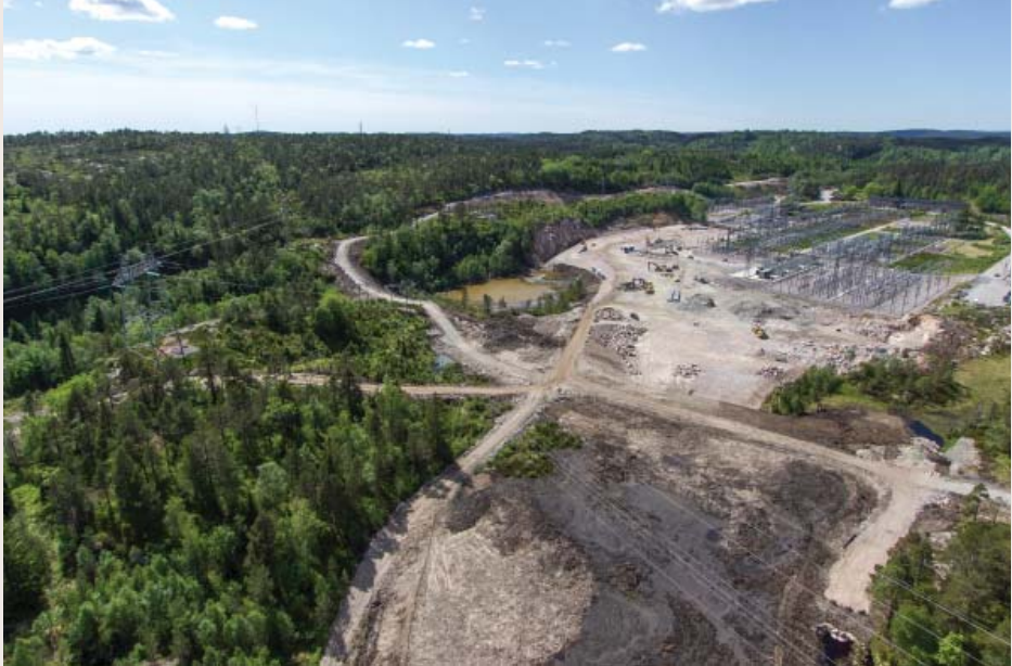
Figure 41 In some situations, it can be necessary to seed an area in order to speed up the re-vegetation. In this situation, a peat landfill (bottom right) was seeded in order to help stabilise the fill material.
